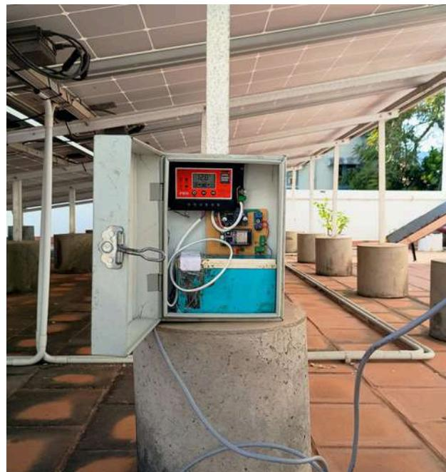
We have successfully installed our newly designed **rain gauge**, a device used to measure rainfall and track precipitation patterns. This upgraded version features an improved battery and wireless connectivity, with ongoing testing to ensure stability and accuracy. Additionally, a low-cost commercial rain gauge has been procured and will soon be deployed in strategic locations across Puducherry for broader data collection and analysis.
