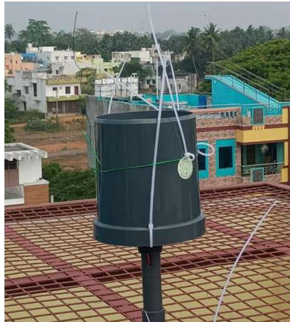
A rain gauge is a simple scientific instrument used to measure the amount of rainfall over a specific period. It typically consists of a cylindrical container that collects rainwater, allowing for accurate recording of precipitation levels. This data is crucial for understanding local weather patterns, planning agricultural activities, and improving water resource management.
